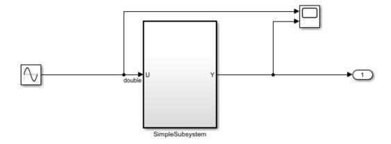
This introductory model shows the code generated for a simple subsystem consisting of a few basic Simulink blocks. To build the subsystem, right-click on the subsystem block and select PLC Code > Generate Code for Subsystem.
