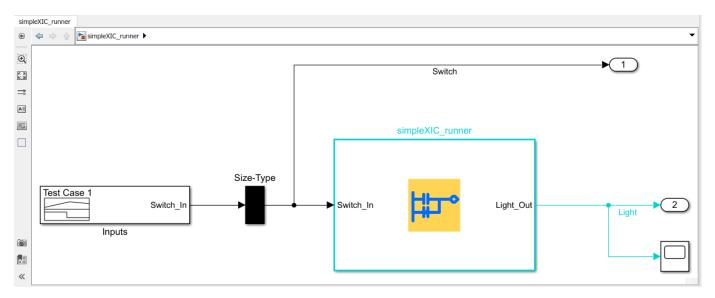
Modify the Signal Builder input to mimic a switch operation as shown.
